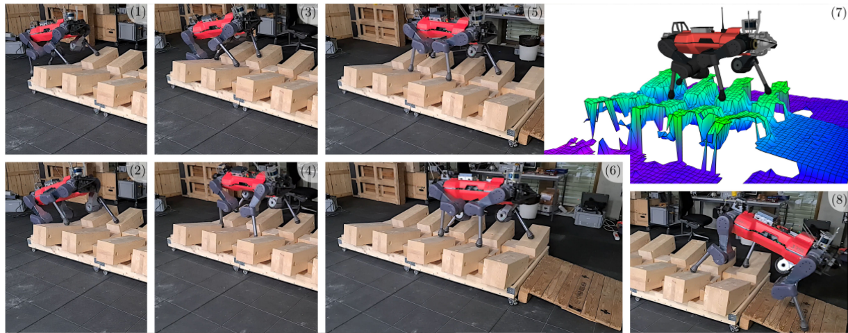
Fig. 19. Anymal traversing a stepping stone parkour made of inclined wooden bricks using a trotting gait. The commanded heading velocity is 0.4 m/s. The dimensions of each brick are 20 cm \times 20 cm \times 50 cm and the gap between any two adjacent bricks measures 20 cm. Due to the inclined surfaces, the model assumptions are not perfectly satisfied in this experiment. (7) Visualization of the robot along the raw elevation map.
